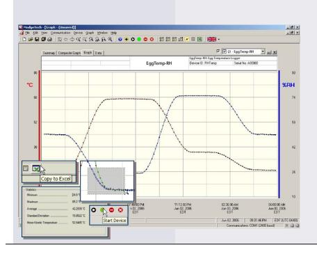
MadgeTech Data Recorder Software displays temperature and humidity data in an easy to use graph.
